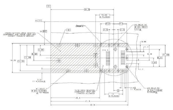
Detum and Basic Dimension Established by Customer Rads and Vias are Chassis Ground, 11 Places Chrough Holes are Unplated
